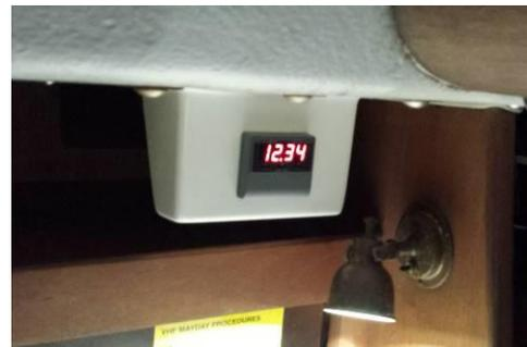
Better still, it can be switched to display amps flowing from the batteries. This took the guesswork out of estimating the amps consumed by different systems on the boat. We learned that the current draw from the following things was:
